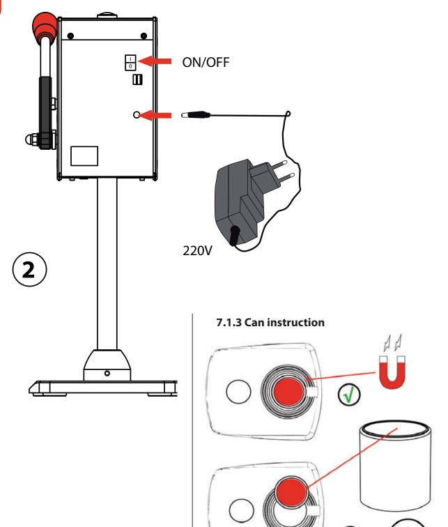
Fill the can **WITH THE SPINDLE IN IT** to 1 cm below the rim.
